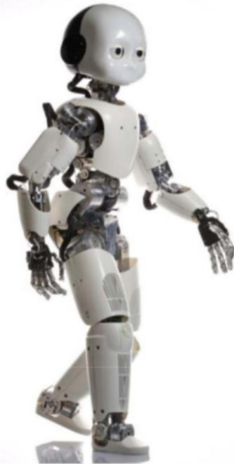
The **iCub** is the humanoid baby-robot designed as part of the **RobotCub** project
