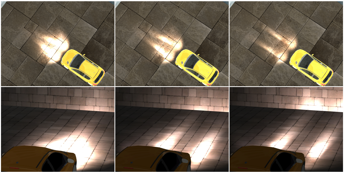
Fig. 14. Light editing for car2 headlight data. Our technique allows to modify interactively (8fps in average) the position and orientation of captured light field.
