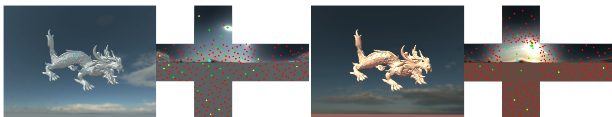
Figure 1: Time-varying light samples distribution for one pixel (cyan dot) on the dragon model when lit with a dynamic environment map [STJ*04]. In the cube map images, the cyan dot corresponds to the normal direction. For each frame, among on-the-fly generated samples (red+yellow+green) on the whole environment map, our technique selects 50 of them (yellow and green dots). The green dots correspond to effective samples where the cosine factor is strictly positive. At nearly noon ( Left ), our technique selects less samples on the sun than at sunset ( Right ), since it is located at a more grazing angle. This example runs in average at 145 fps using Multiple Importance Sampling with 50 samples for the energy conserving Lafortune Phong BRDF with a shininess exponent set to 150.
