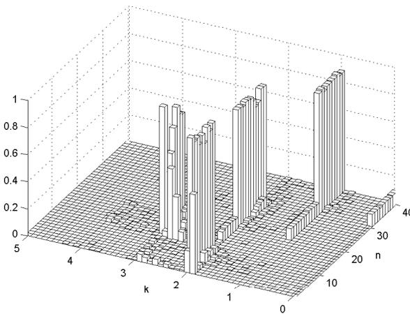
Figure 4. Auxiliary particle PHD filter. Estimated number of targets averaged over 200 observation realisations.
