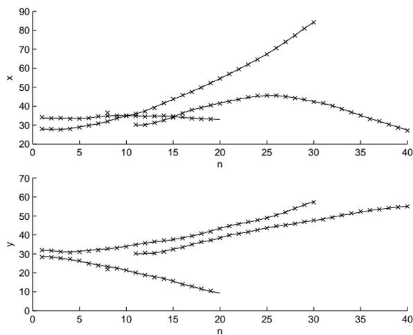
Figure 2. Ground truth target positions (solid line) and state estimates (crosses) for auxiliary particle PHD filter.
