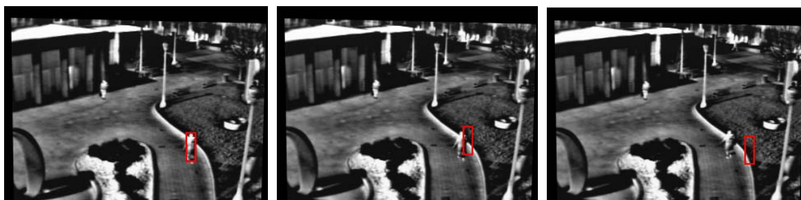
Figure 9. Tracking results for frames No. 1, 5, 10 in sequence #1 using algorithm 2.
