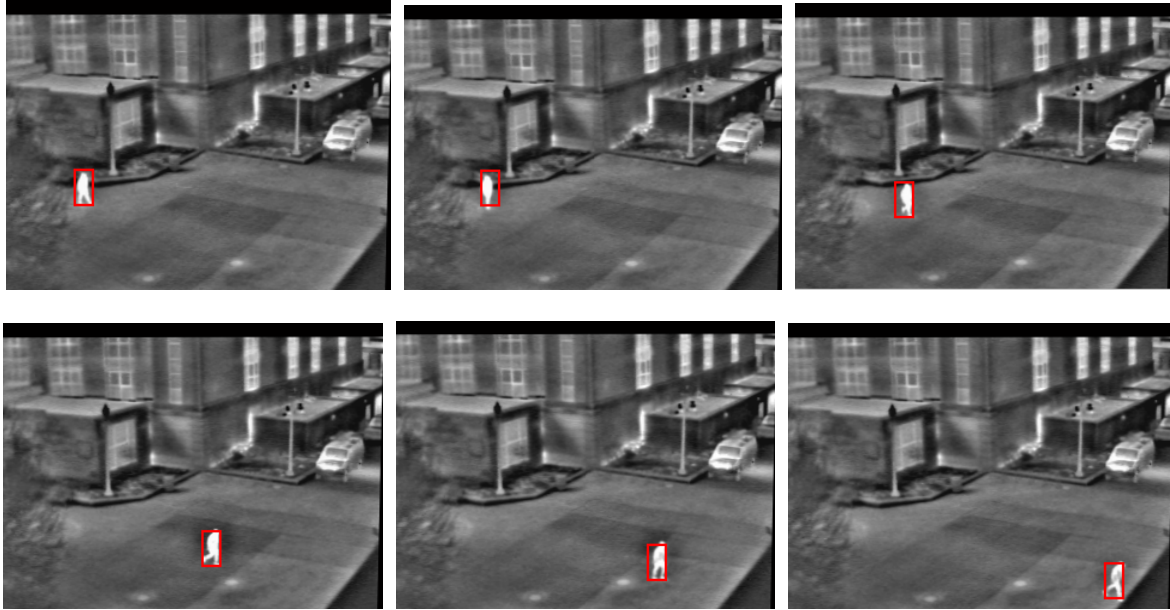
Figure 10. Tracking results for frames No. 1, 10, 50, 150, 200, 250 in sequence #2 using algorithm 1.
