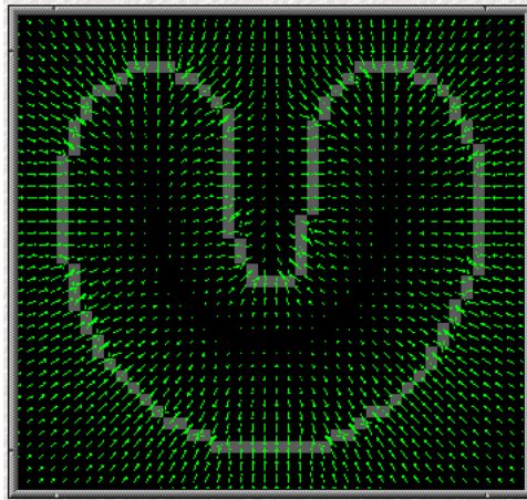
Figure 2.2 The gradient vector flow (GVF) external force field for a U-shaped object 11 .
