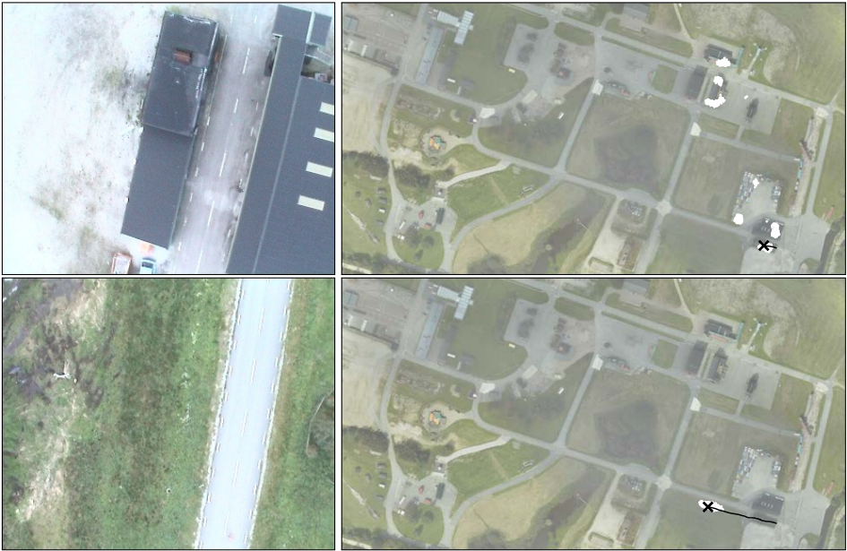
Figure 1.3: Top row - Image from the on-board camera (left) and particle positions (right) after 5 seconds of flight. After having received several images containing asphalt and buildings, the number of possible positions of the UAV is drastically reduced. Bottom row - Image from the on-board camera (left) and particle positions (right) after 20 seconds of flight. Once the UAV proceeds along one of the roads, the remaining faulty hypotheses can be discarded since they do not match the images obtained from the camera. The true vehicle position is shown as a black cross and the vehicle trajectory as a solid line.
