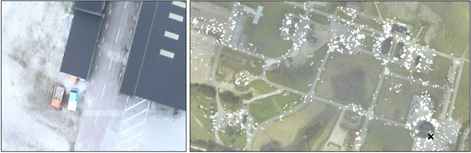
Figure 1.2: Image from the on-board camera (left) and particle positions (right) after 1 second of flight. The image processing system on the UAV detects asphalt and buildings in the image. Hence, several of the initial hypotheses can be discarded since they do not match the image. Instead, focus is put on areas along the roads and especially near the buildings.
