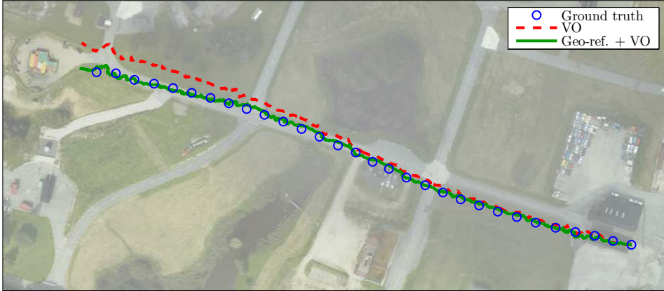
Figure 3.5: True trajectory illustrated with circles and the estimated trajectories with (solid line) and without (dashed line) geo-referencing.
