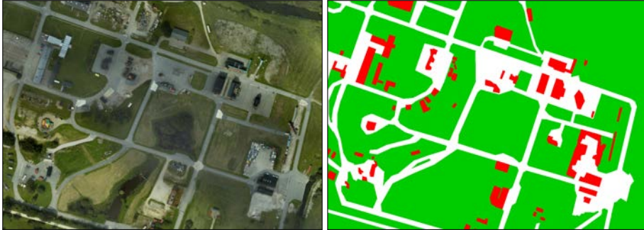
Figure 3.2: Map over the operational environment (left) and a manually classified reference map with grass, asphalt and houses as prespecified classes (right). Aerial photograph by courtesy of the UAS Technologies Lab, Artificial Intelligence and Integrated Computer Systems Division (AIICS) at the Department of Computer and Information Science (IDA), Linköping University, Linköping, Sweden.
