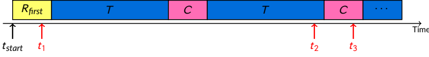
FIGURE 16 Illustration of the notations for the victim job, with the five cases distinguished to compute the future checkpoint strategy (T3).
