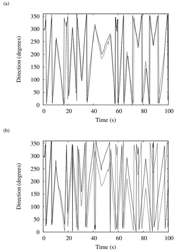
Figure 12: Tracking of the robot actual direction (represented by the dashed line) by the MT9 device (a) and by the integration of the input from the odometers (b).
