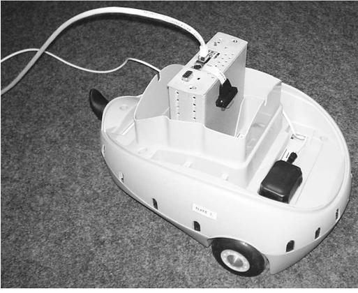
Figure 3: The mobile Pekee robot with the MT9 device (the black box in front of the robot) for sensing inertial self-motion signals.
