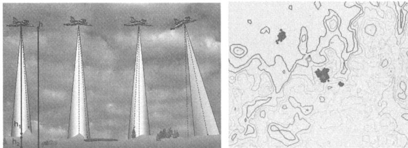
Fig. 16. Left figure is an illustration of an aircraft measuring distance  $h_1$  to ground. Onboard baro-altitude supported INS system provides absolute altitude over sea level  $h$ , and difference  $h_2 = h - h_1$  is compared to a topographical map. Right plot shows a snapshot of PF particle cloud just after aircraft has left sea in upper left corner. There are three distinct modes, where the one corresponding to the correct position dominates.
