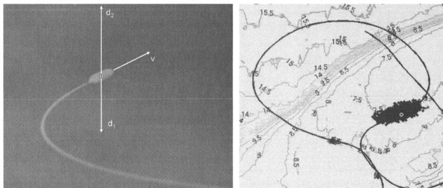
Fig. 13. Left plot is an illustration of UW vessel measuring distance  $d_1$  to sea bottom, and absolute depth  $d_2$ . Sum  $d = d_1 + d_2$  is compared with a bottom map as illustrated with contours in plot to right. Particle cloud illustrates snapshot of PF from known validation trajectory in field trial, see [75].
