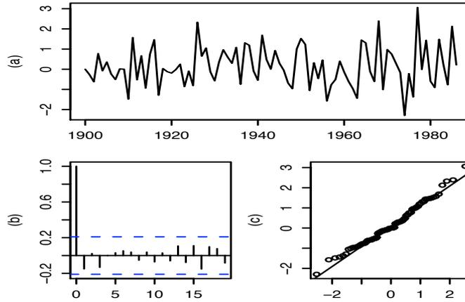
**Fig. 3.4.** (a): Standardized one-step-ahead forecast errors; (b): ACF of one-step-ahead forecast errors (c): Normal probability plot of standardized one-step-ahead forecast errors
