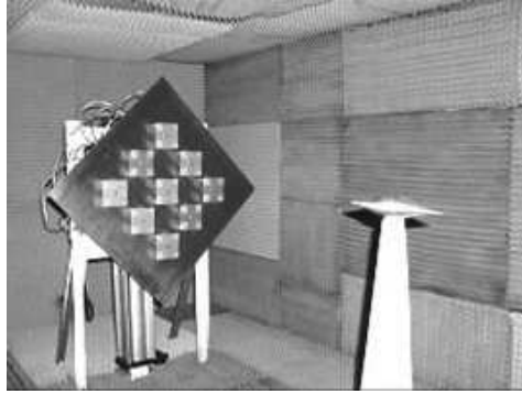
Figure 1. RCS measurement inside an anechoic chamber
