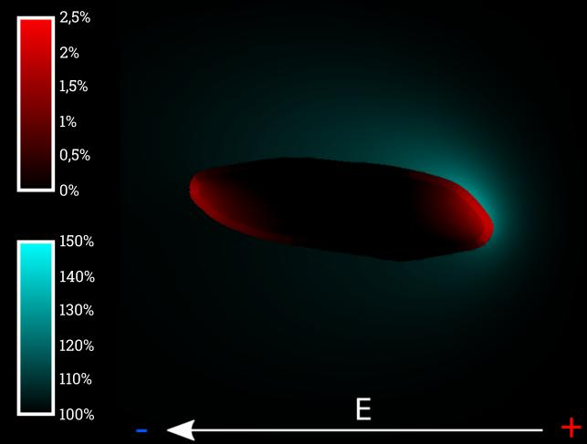
2D Simulation of PI transport (without lipid diffusion) for a cell submitted to the same pulse protocol as used by Vernier *et al.* in [5] : five pulses of 100 µs, 500 kV/m, 4Hz. The indicated times start at the end of the last pulse. Same color scale as to the left. >
