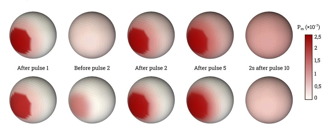
Permeabilization  $P_m$  of a cell submitted to 10 pulses of 40kV/mduring 10 µs. The top line corresponds to a time lapse of 1s between pulses and 1ms for the bottom line.
