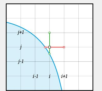
> Numerical schemes : our very irregular mesh induces numerical instabilities for the transport-diffusion equation on M. Thus, a splitting of these two steps is performed. A fixed point method is performed for the diffusion step to capture accuratly the non-linearity of  $P_m$ .
