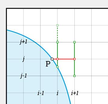
■ Example of flux discretization at interface point P, located left from *ij*:
