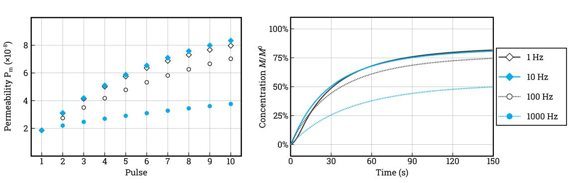
$\blacktriangle$  Averaged permeabilization degree  $P_m$  after each pulse (left panel) and time evolution of the molecule concentration M (right panel), relatively to the external concentration  $M^0$ , for pulse application frequency from 1 to 1000 Hz.
